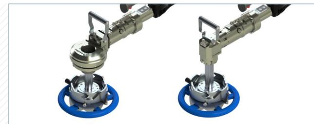
FSB adaptors require the KTA002 interface with a straight or right angle drive head, and the TTA002 interface with a banjo head.
