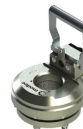
The **Heavy duty banjo drive head** should be used for **very high torques**. It caters for **rising stems up to a maximum diameter of 70mm (2.75")** and is compatible with all clamping systems for handwheel and other interfaces. It brings additional reduction which means you can **multiply the actuator's torque by 3** and reduce the speed by the same factor.
