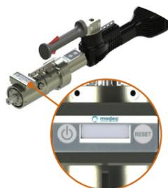
The **digital revolution counter** adds up the turns in one direction and subtracts them in the other direction so that the operator always knows where he is in relation to the starting point. **It also measures and indicates the rotating speed.**
